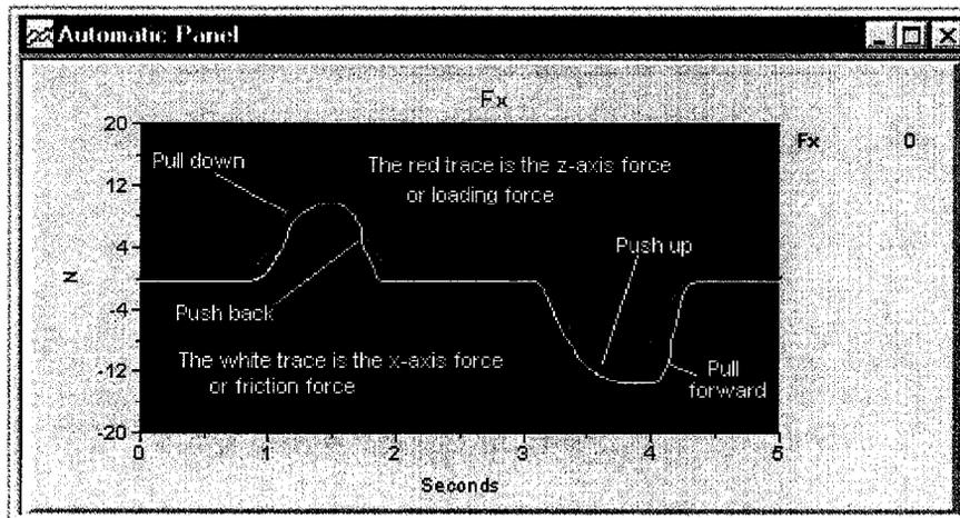
Pulling downward on the suspension should move the **red** trace upward. Likewise, pushing up on the suspension should move the **red** trace downward.
