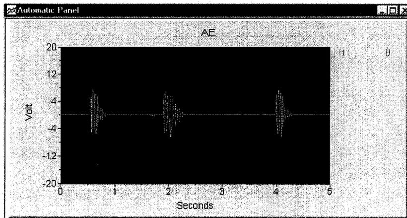
Tap the AE sensor lightly against the body of the tester. Pulses should appear on the real time trace.
