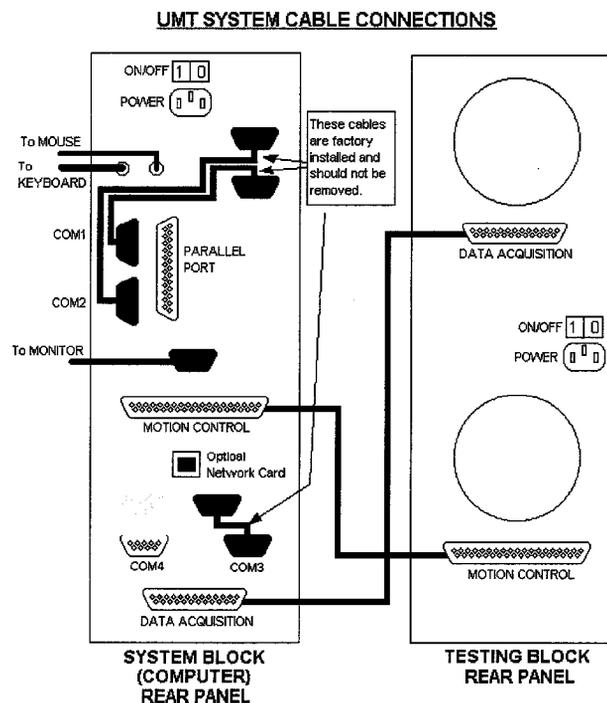
COM1, COM2, and COM3 connectors should already have cables connected. These should be left as is. COM4 may also have a cable if it is a 4 drive system.
