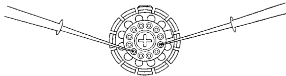
Figure 4-11. Checking for proper electrical connection of the sample
