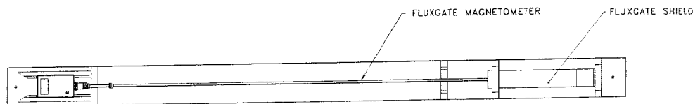
Figure 2-7. VSM ULF storage (wall) bracket and fluxgate magnetometer
