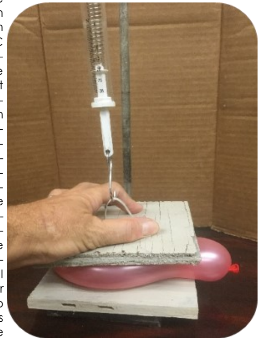
Demonstration of slowly squishing the water balloons to record the force required to break it.
