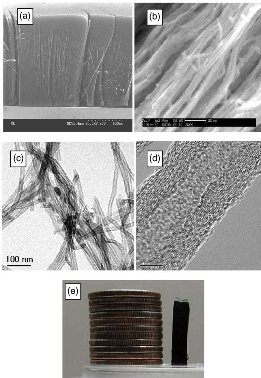
Fig. 1. ESEM images of aligned MWCNT arrays at: (a) low resolution, and (b) high resolution, HRTEM images at (c) low resolution, and (d) high resolution; (e) picture of a MWCNT array with 11 US quarters for size reference. Growth conditions: 200 SCCM of H<sub>2</sub> flow, 200 SCCM of C<sub>2</sub>H<sub>4</sub> flow, 100 SCCM Bubbler flow, 750 °C growth temperature.
