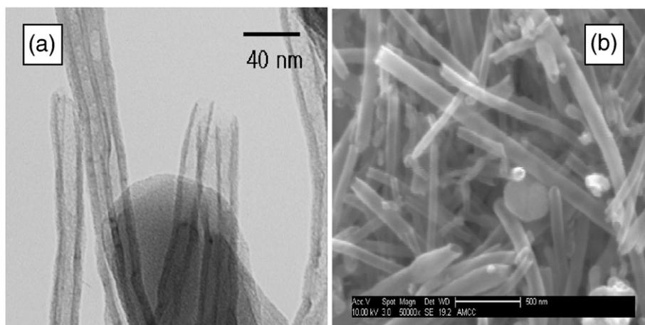
**Fig. 4.** Effect of functionalization: (a) TEM image of functionalized MWCNT; and (b) ESEM image of functionalized CNF.
