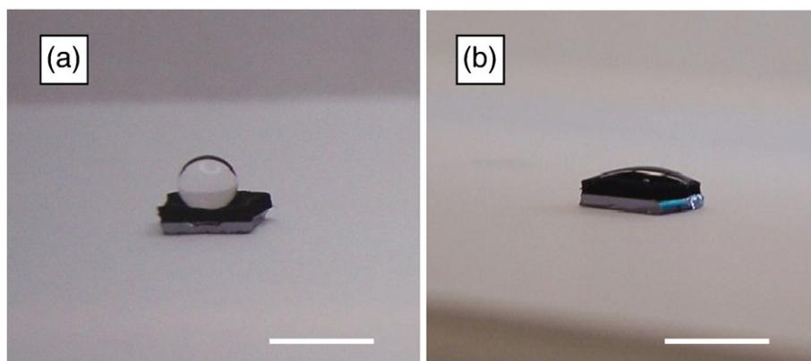
Fig. 3. Images of aligned multi-wall carbon nanotube carpets: (a) photo of a water droplet on a 1 mm long nanotube as grown array, and (b) array after functionalization using acid showing wetting of the surface. Bar is 1 cm.
