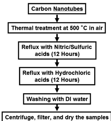
Fig. 2. Functionalization steps for MWCNTs and CNFs for use in cell culturing.
