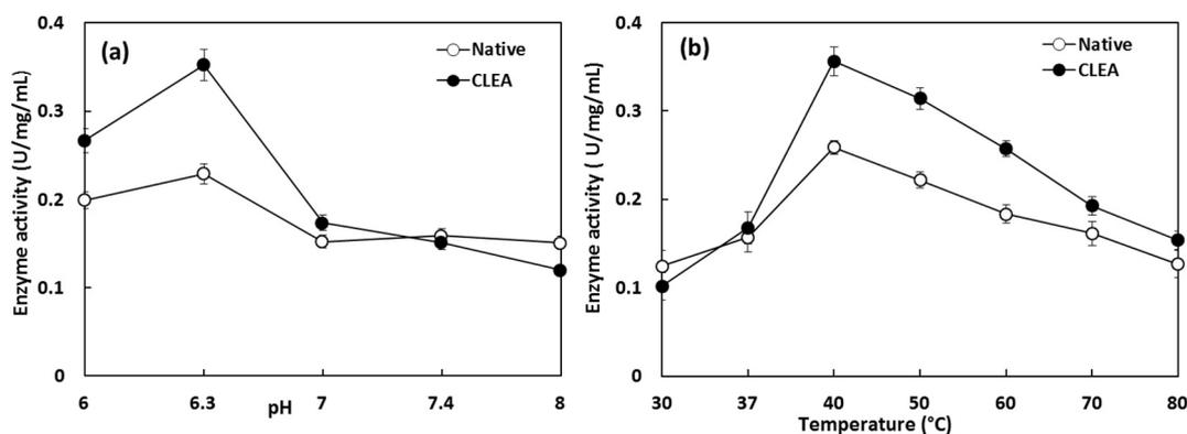
Fig. 3. (a). pH profile of native alginate lyase (1 U) and CLEA-AL (1 U) in phosphate buffer (pH 6–8); (b) temperature profile of native (1 U) and CLEA-AL (1 U) in phosphate buffer (temperature 30–80 °C).
