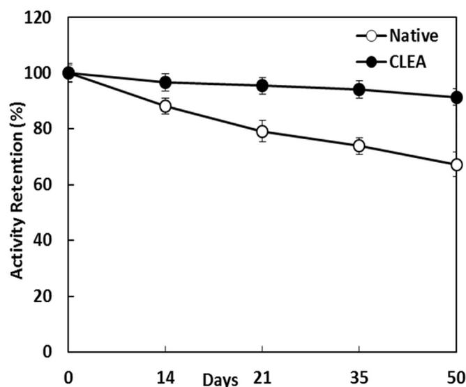
Fig. 6. Storage stability of free and CLEA-AL (1 U) at 4 °C.
