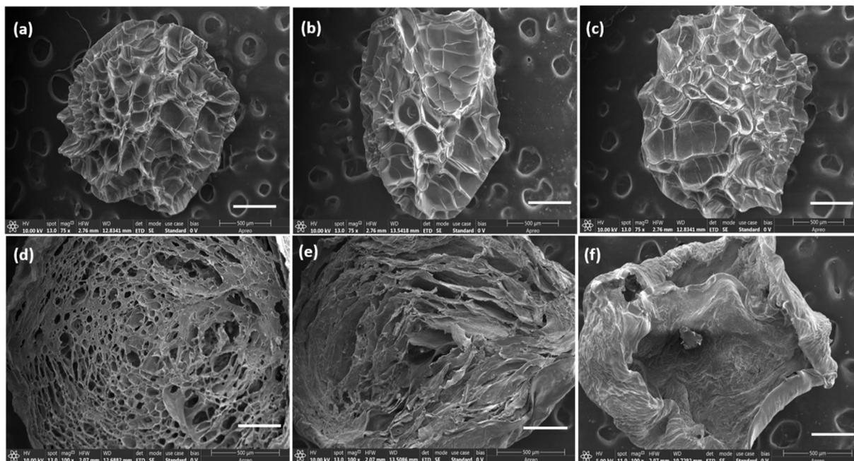
Fig. 7. SEM images of hydrogel beads with (a) control hydrogel (0 U); (b) native enzyme (1 U) and (c) CLEA-AL (1 U) incorporated; (d) cross sectioned control; (e) cross sectioned native and (f) cross sectioned CLEA-AL incorporated (scale bar  $500 \mu\text{m}$ ).
