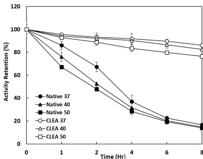
Fig. 4. Thermal stability of native (1 U) and CLEA-AL (1 U) at 37°, 40°, and 50 °C with time.
